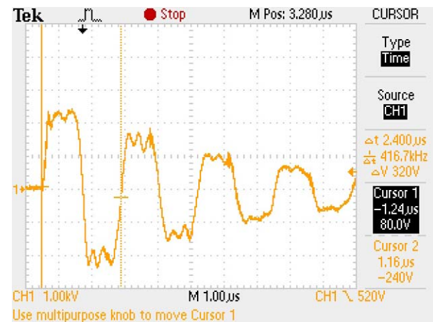
Fig. 2 Bipolar square waveform across electrodes in water sample.
