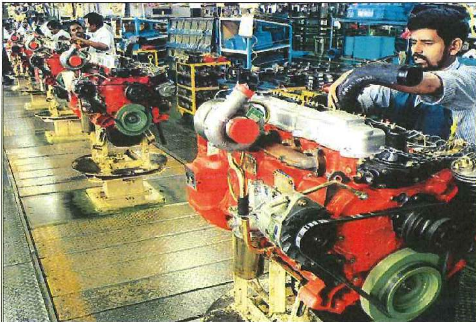
Fig.2 Engine assembly section
