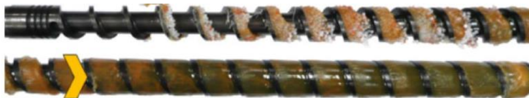
Fig 2.6 Distribution of melted and solid materials in the screw (a) Starve feeding (b) Flood feeding
